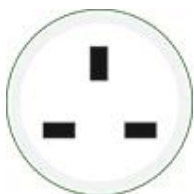
stekker/ stopcontact: BS 1363 (British)
