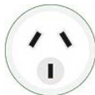
stekker/ stopcontact: AS/NZS 3112 (Australian)
